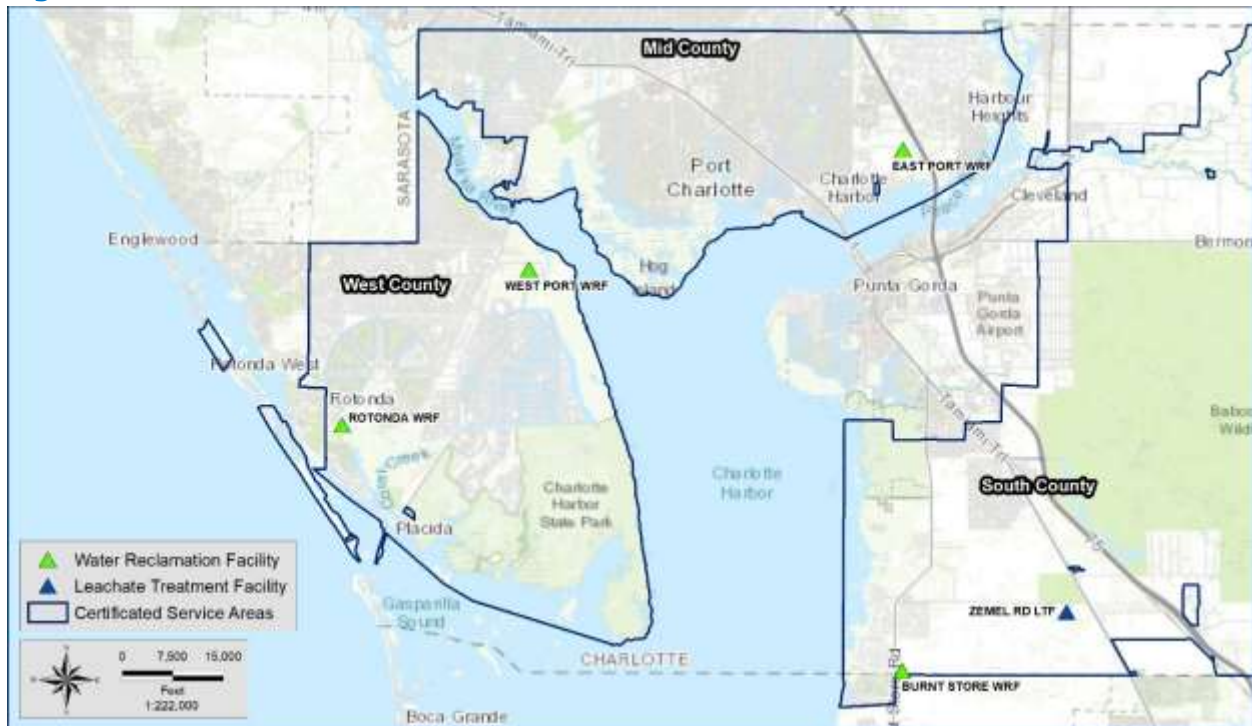
Figure 6-1 CCU Wastewater Treatment Facilities
